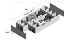
A strategy that adopts a modular cleanroom pod approach enables maximum flexibility for GMP modules to be added at speed to support additional dose capacity.
